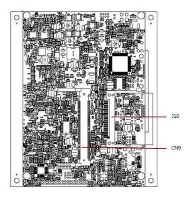
Figure 3-2 Locating Jumpers and Connectors on Panel PC (rear side)
