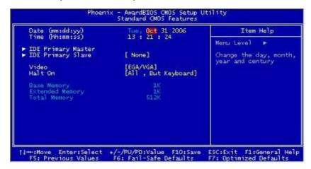
Figure 7-2 Standard CMOS Features
