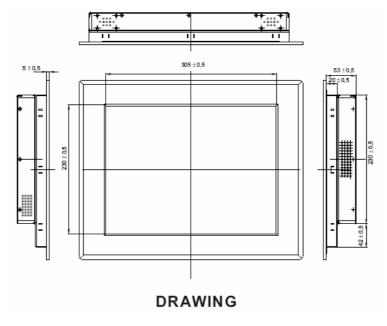
Figure 1.19 15" Mechanical Drawing
