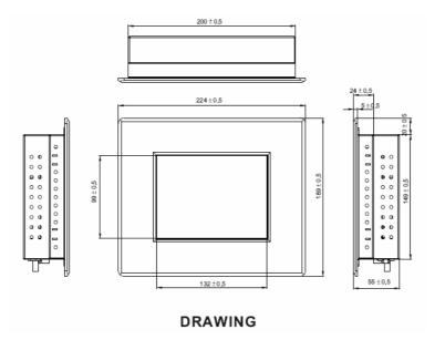
Figure 1.4 6.4 " Mechanical Drawing
