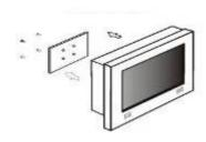
Fix the Panel PC with four screws (standard VESA), and fasten to the wall with other four screws.
