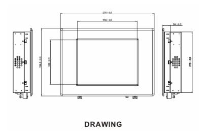
Figure 1.10 8.4 " Mechanical Drawing
