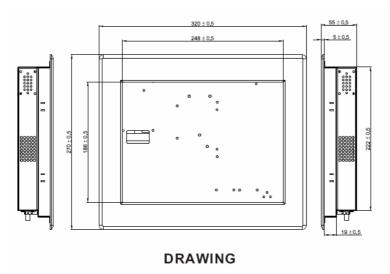
Figure 1.16 12.1 " Mechanical Drawing
