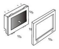
Fix the Panel PC to the supporter with mounting kit, and affix the front frame to the panel with screws.
