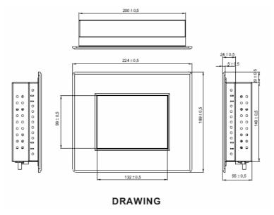
Figure 1.7 6.5 " Mechanical Drawing
