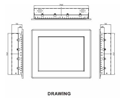
Figure 1.13 10.4 " Mechanical Drawing
