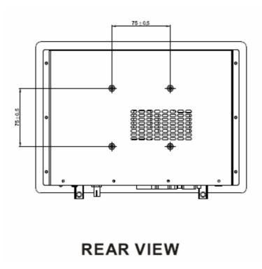
Figure 1.8 8.4 " Mechanical Rear View
