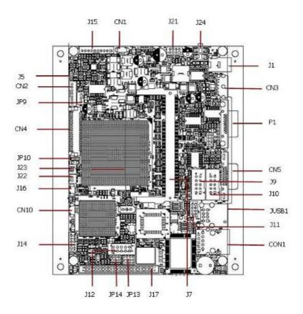
Figure 3-1 Locating Jumpers and Connectors on Panel PC (front side)
