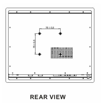
Figure 1.14 12.1 "Mechanical Rear View
