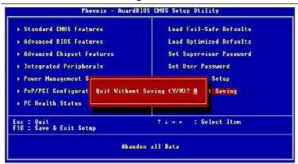
Figure 7-10: Exit without Saving setup screen
