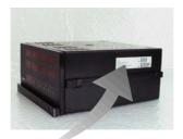
An identification plate is glued on the controller housing. The information on this identification plate enables you to determine the delivery condition from the factory as well as the date of manufacture of the controller.
