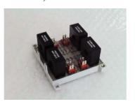
Current acquisition card for exact acquisition of up to 4 single-phase heating circuits.
