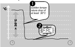
If the setpoint value > actual value during the FAL response time and with max. possible degree of control (observe possible degree of control limitation) does not lead to a temperature rise of at least 4°C, the FAL alarm will be initiated.
