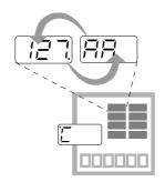
During the automatic starting adaptation (cooling) the zone display will show AA- alternately with the actual temperature value.
