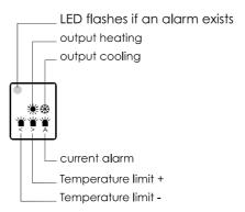
The LED in the acknowledge key will only flash if at least one alarm in a zone exists.
