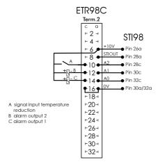
Use of controller internal power supply voltage
