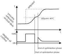
The heating control parameters are calculated from the dynamic behaviour of the actual value process and from that the cooling parameters are derived. The data is stored in the EEPROM and overwrite the control parameters previously used.
