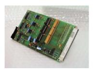
Current acquisition card in Euro card format for processing of up to 8 three-phase heating circuits.
