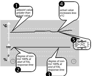
With identification of one of the two operating conditions the alarm will be initiated and the respective zone made passive. Re-activation of the zone will only take place after acknowledgment of the alarm.
