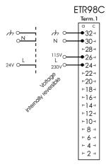
Fusing for the controller must be fitted externally.
