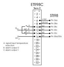
External power supply voltage for alarm outputs and depression input
