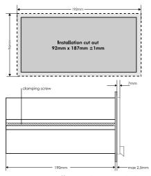
Ensure that there is sufficient clearance behind the controller to accommodate the wiring
