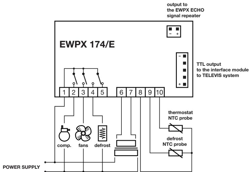
**Remote connection:** serial connection to the EWPX ECHO repeater (version /E only).
