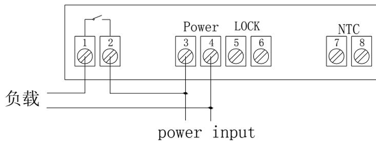
Load and temperature control use the different power adapter
