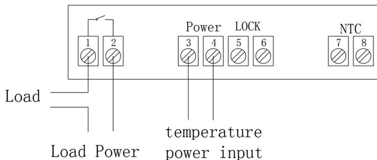
Terminals 1 and 2: Normally opened contact of relay
