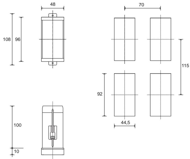
Dimensions: 48x96mm (1/8DIN), depth 100mm
